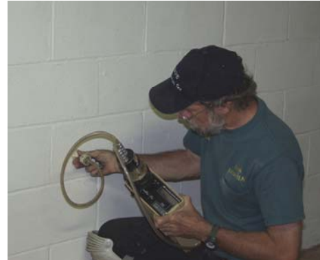
Fig 3-26 Radon sniffer checking block wall
