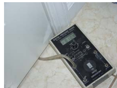
Fig 3-22 checking basement pressure
