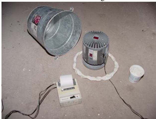
Fig 4-8 Slab flux test
